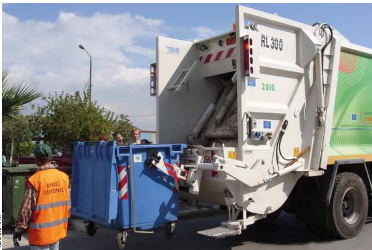
Refuse collection lorry with weighing equipment
