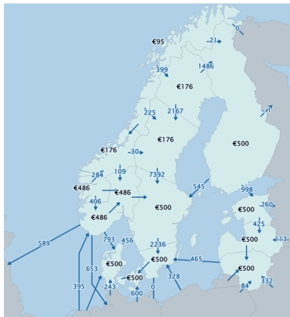
Figure 1: Map of electricity prices (in EUR/MWh) and flows (in MWh) at 17:00, December 15 th , 2022. Source: Svenska Kraftnät ( https://www.svk.se/om-kraftsystemet/kontrollrummet/ ).
