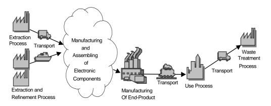
**Figure 6** A schematic description of the access of LCI data in the production chain of electronic components. The cloud implies that the access of data regarding the manufacture and assemblage of components is scarce.
