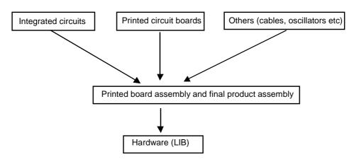
Figure 8 The LCI model, developed at Ericsson Enterprise Systems, shows how the components included in a line interface board (LIB) are divided into three LCI-data groups. Further, the assembly can be added in the model.
